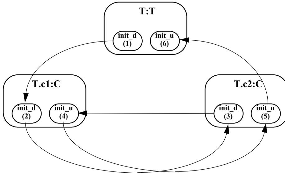
Figure 18—Order of invocation of `init_down` and `init_up` exec blocks
